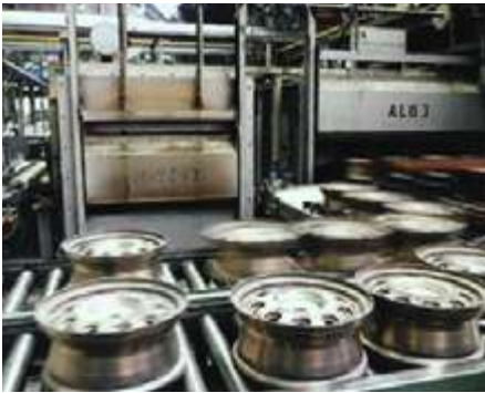
Aluminium industry: curing oven for wheel rims
