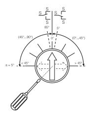
Switch a factory-set at 5°. The auxiliary switch can be optimally adjusted between 0°...90°.
