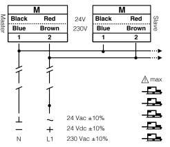
Parallel connection of maximum five MDS actuators is possible. The power consumption must be observed.
