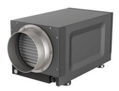
**Pipe Size:** In the case of the pipe length does not exceed 25 feet, please use a round pipe with a diameter of at least 8 inches; In the case of the length of the pipe exceeds 25 feet, please use a round pipe with a diameter of at least 10 inches. If there are two-three pipe branches at the main inlet/outlet, please use a round pipe with a diameter of at least 8 inches. If the main inlet / outlet has 4 or more pipe branches, please use a round pipe with a diameter of at least 10 inches.
